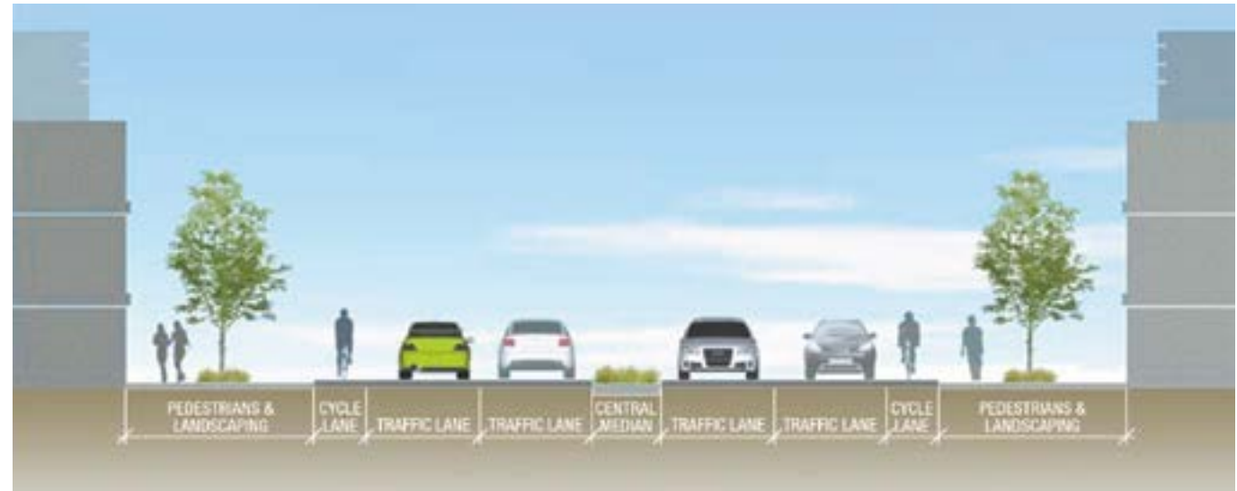
Figure 16 Indicative cross section – Manning Road
