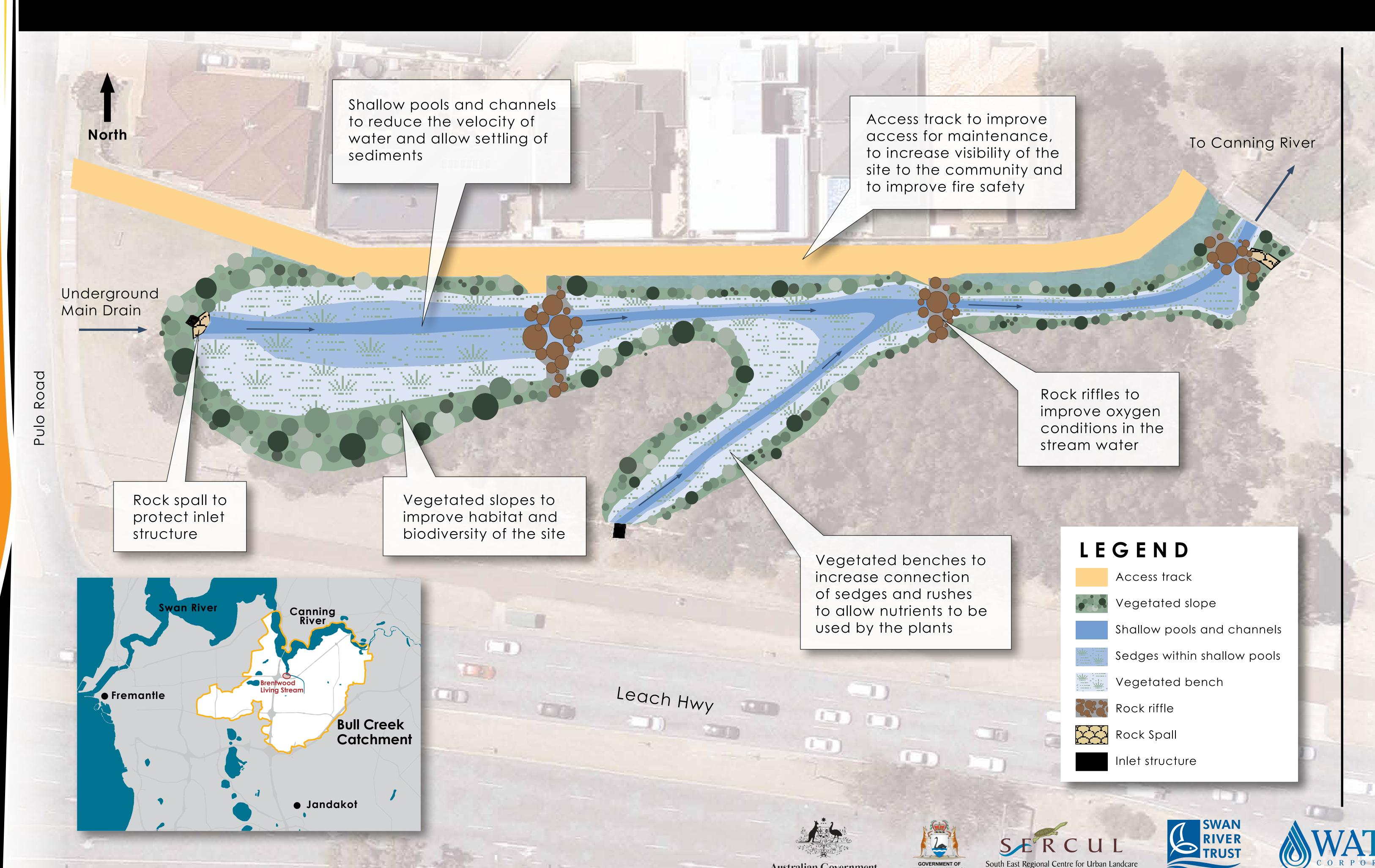
The construction and revegetation works at this site will transform the Brentwood Main Drain and Mandala Crescent Branch Drain into a living stream.
