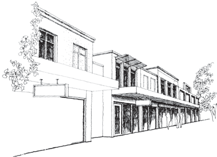
Diagram 1 – Example of high levels of architectural articulation and a differentiated design between the ground floor level and the upper floor.
