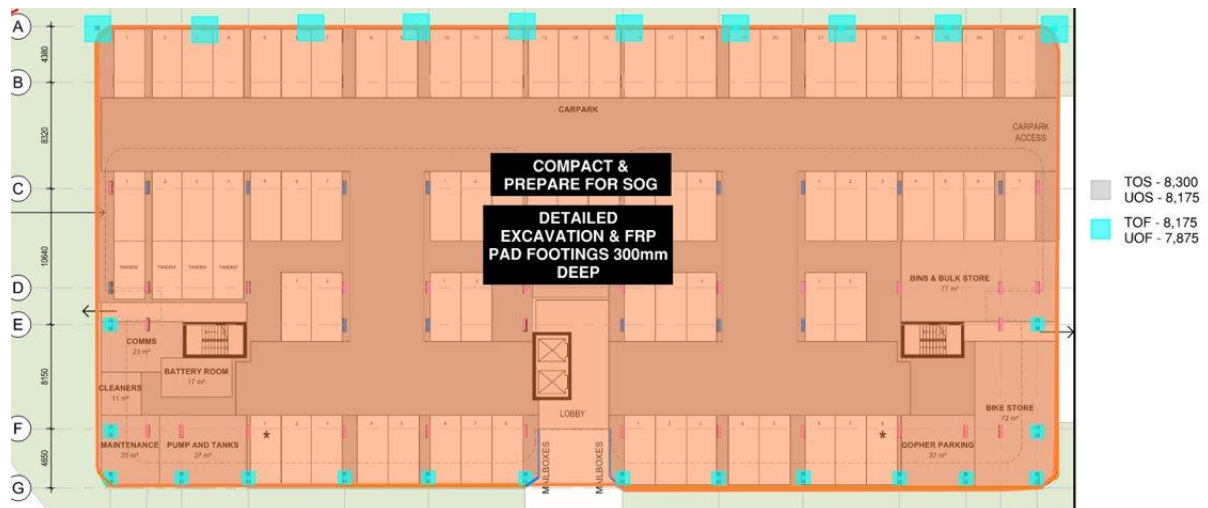
Figure 9: Small Pad Footing Detailed Excavation
