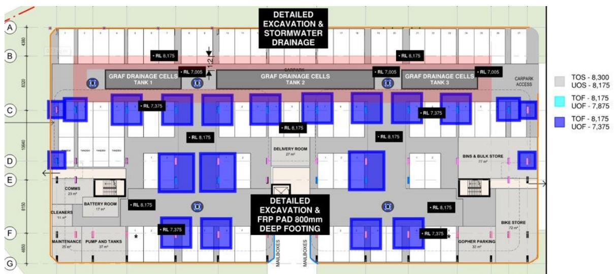
Figure 8: Main Pad Footing Detailed Excavation
