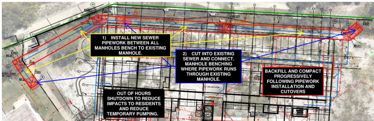
Figure 6: New sewer services continued
