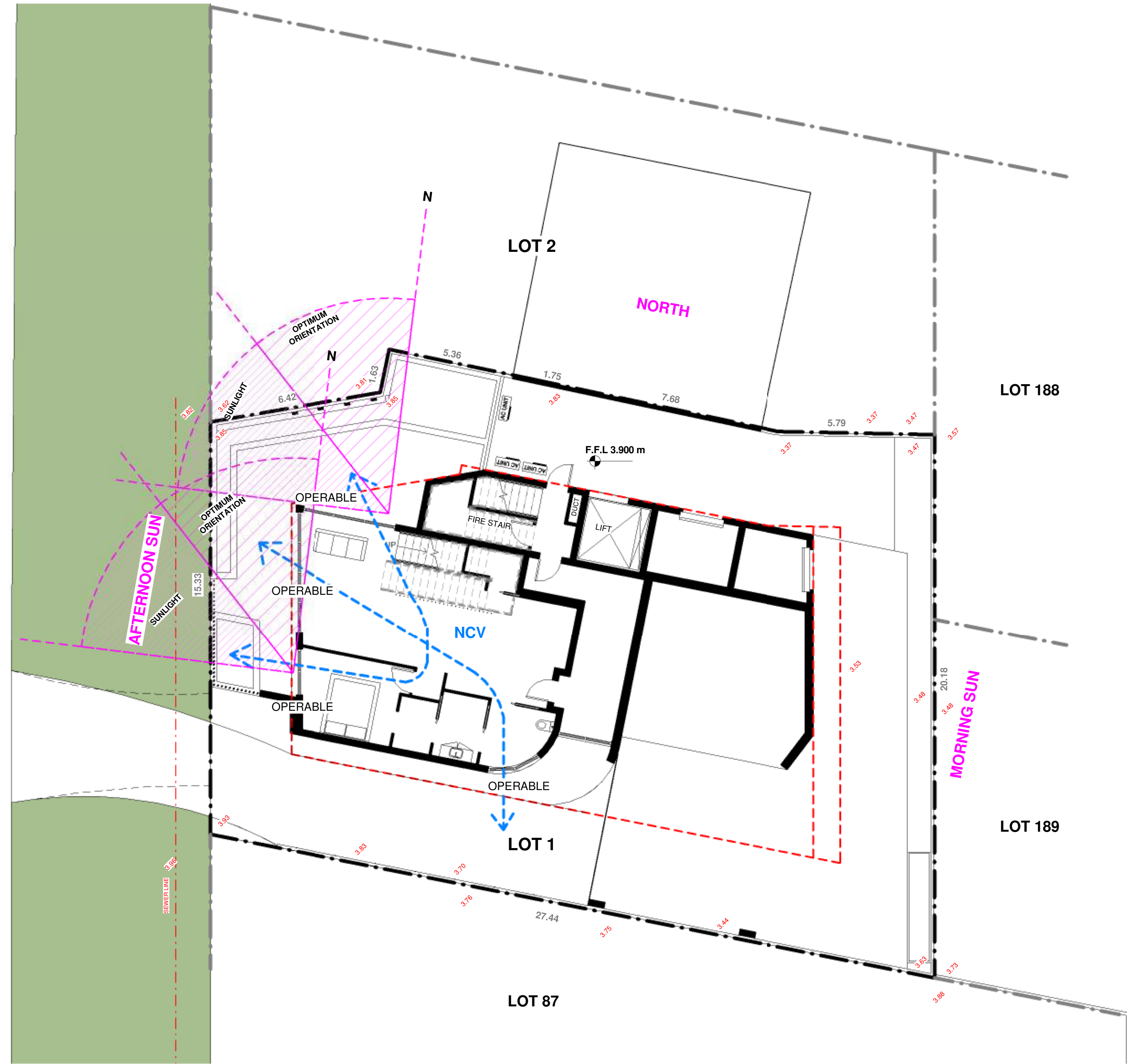
1. SOLAR ACCESS & CROSS VENTILATION DIAGRAM - GROUND FLOOR 1 : 100
