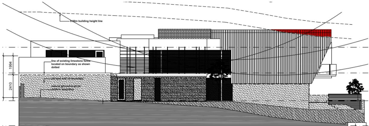
The above diagram depicts the portion of wall which is over height (RED) on the eastern elevation.
