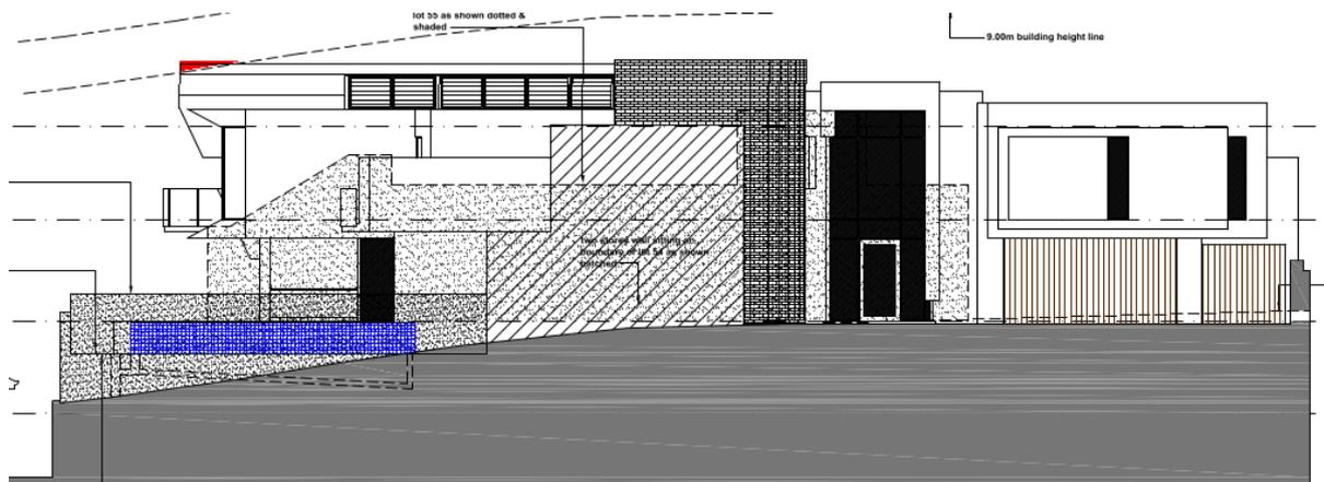
The above diagram depicts the portion of wall which is over height (RED) on the western elevation.
