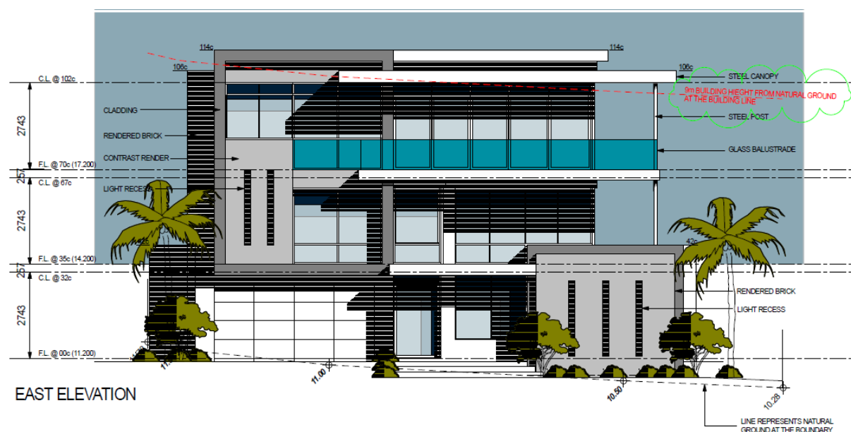
Figure 1. East elevation of proposed development (9.0m building height indicated by dashed red line).
