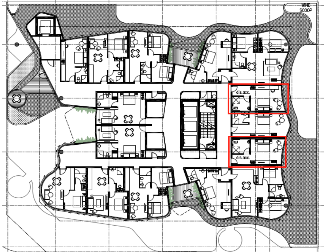
Figure 20: Proposed Level 2 with 15 short stay accommodation units comprising 5 x studio, 5 x 1 bedroom and 5 x 2 bedroom units. 2 units now provided as dible accessible units as marked in red
