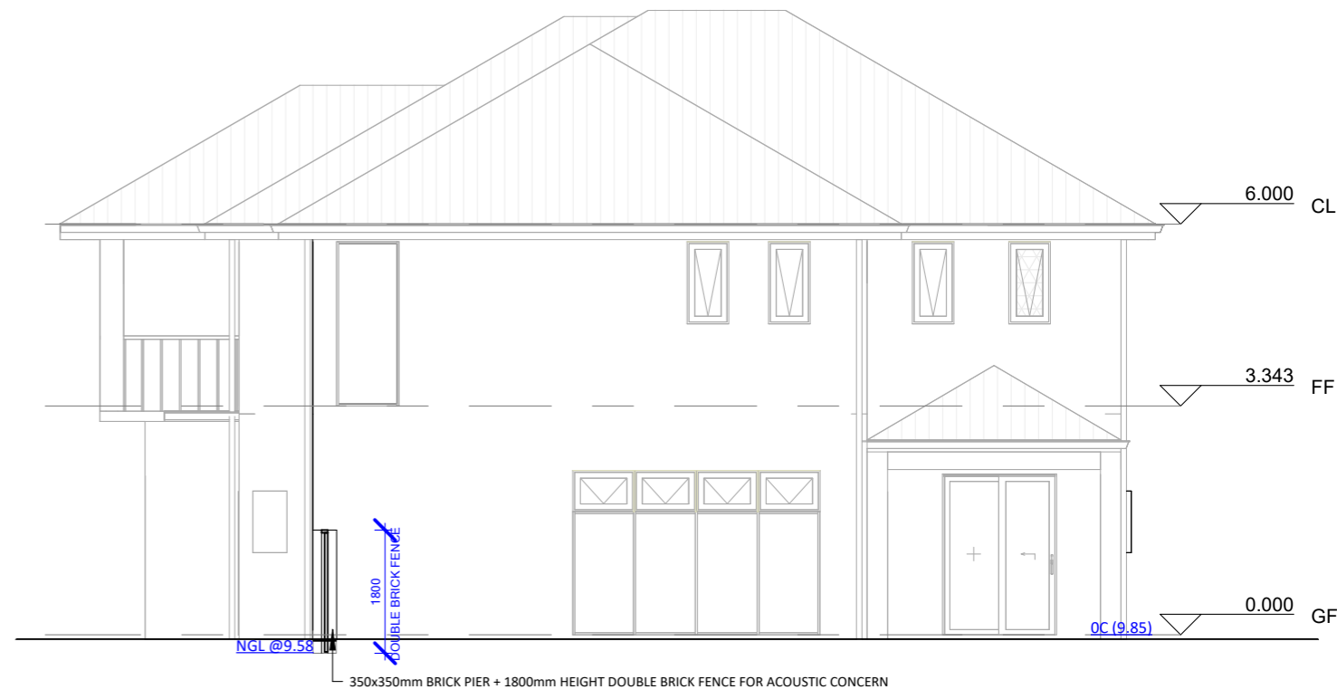
2 FENCE ELEVATION 2 A202 1 : 100
