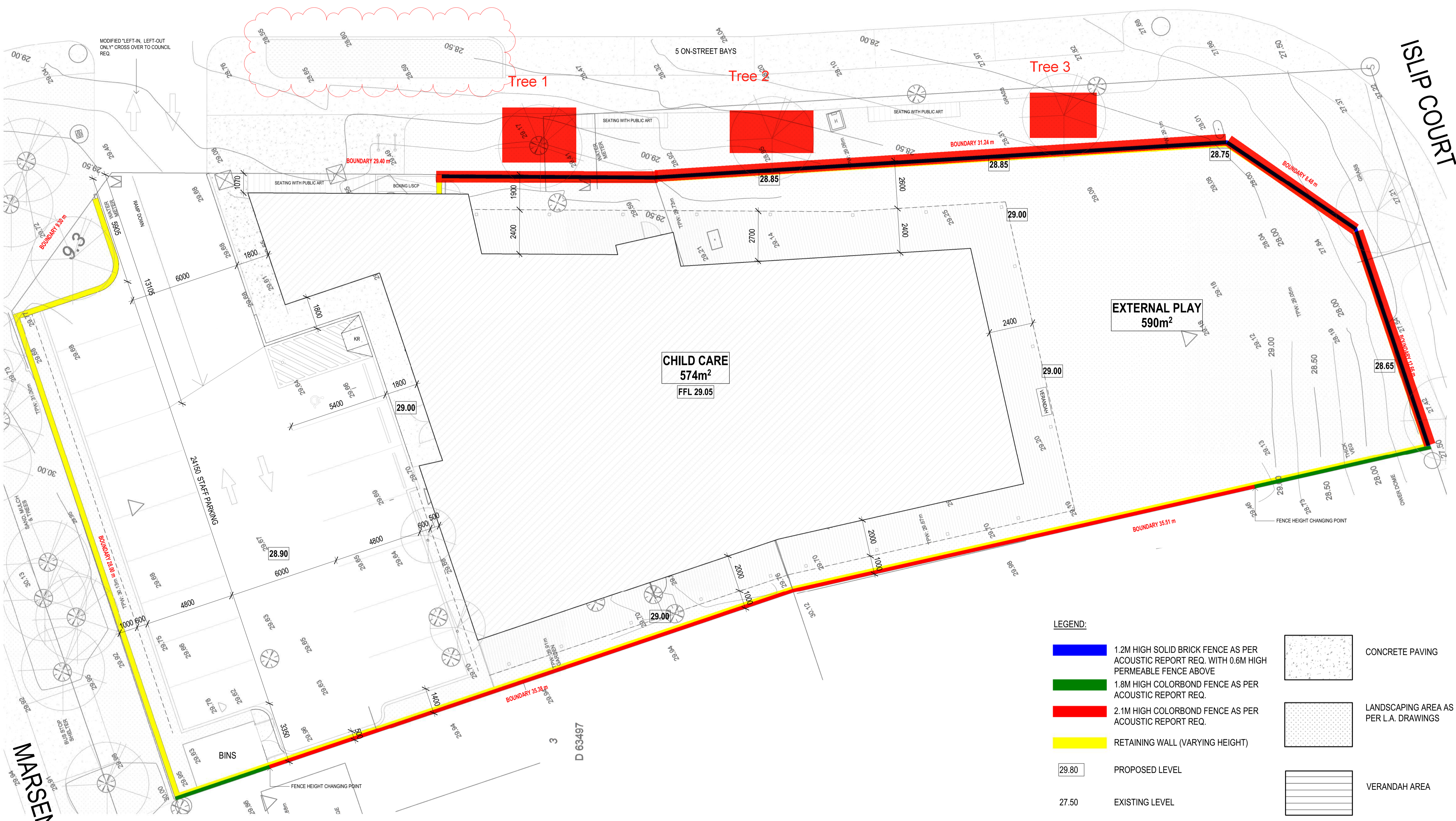
1 ACOUSTIC FENCE AND RETAINING WALL PLAN 1:100
