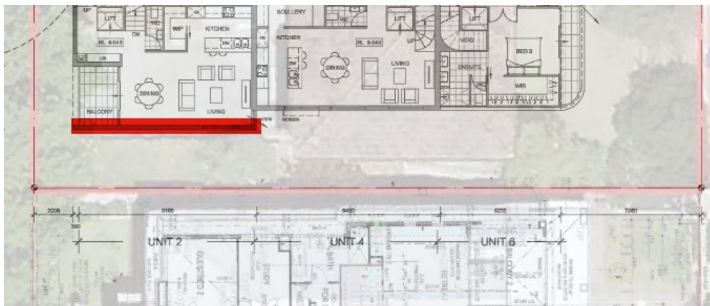
Figure 11: Second floor plan of the proposed development and its relationship with 2B Tweeddale Road. The setback variation is highlighted in red
