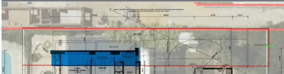
Figure 3: Portions of the first floor within the setback area are highlighted in blue
