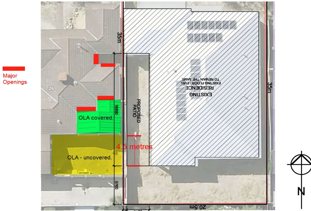
Figure 2: Image showing the outdoor living area and major openings to habitable rooms (marked in red) at No. 26 McGillivray Gardens in relation to the proposed patio.
