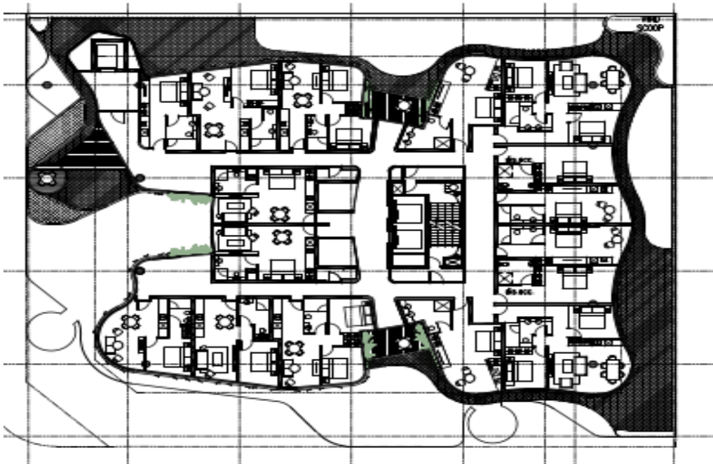
Figure 21: Current Level 2 plan with 16 short stay accommodation units comprising 7 x studio, 5 x 1 bedroom and 4 x 2 bedroom units with 2 units still being disable accessible units
