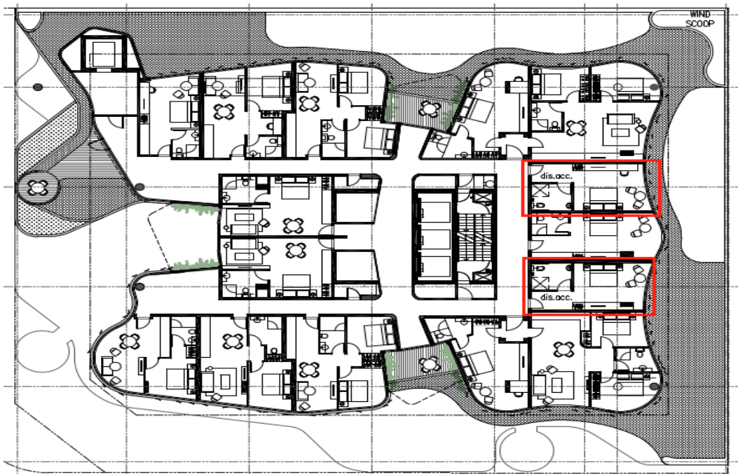
Figure 20: Previous Level 2 plan with 15 short stay accommodation units comprising 8 x studio, 3 x 1 bedroom and 4 x 2 bedroom units with 2 units marked in red being disabled accessible units
