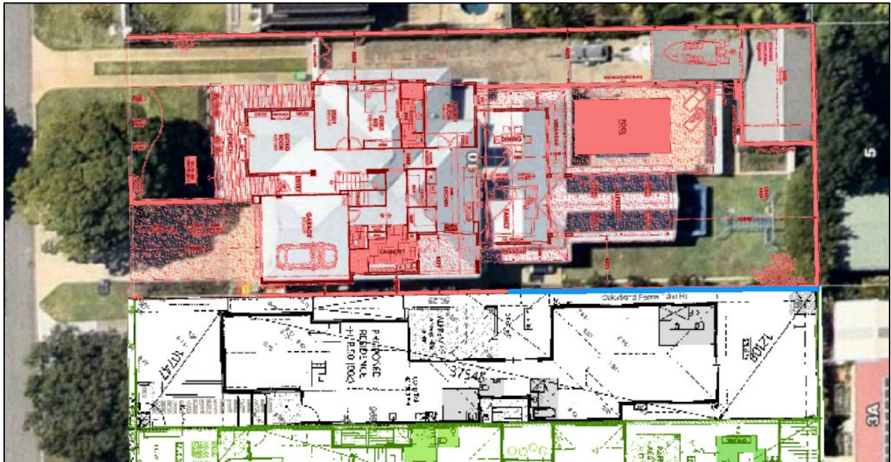
Figure 3: Aerial image with site plan overlay for 10 Birdwood, 8B Birdwood, and 8A Birdwood. The area which is more than 0.5m above natural ground level is highlighted blue.
