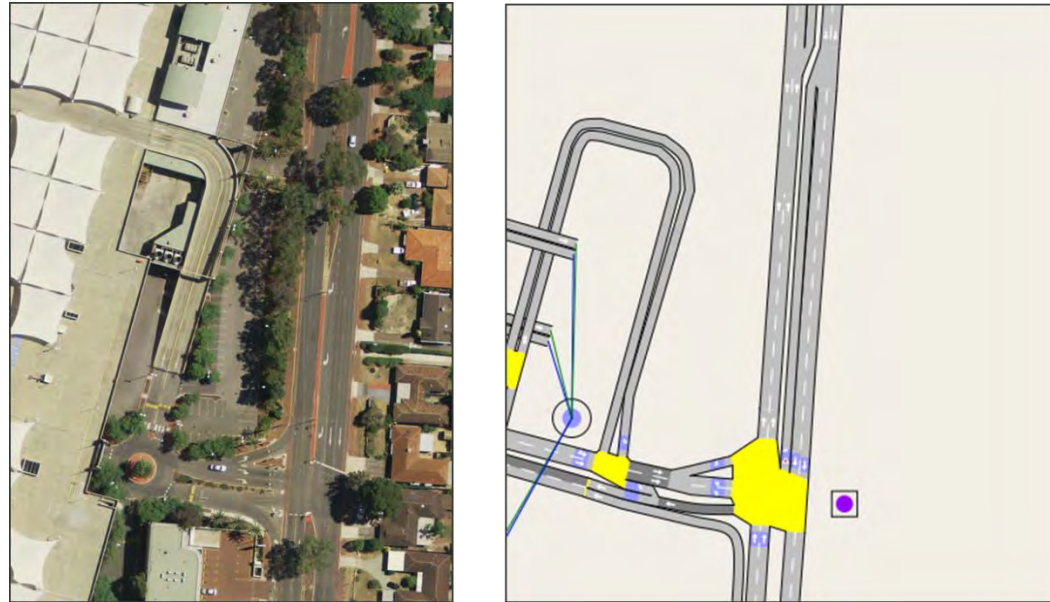
Figure 27 - Proposed upgrade of Riseley Street / Garden City access intersection The width and extent of the median will be reduced to accommodate these proposed works.
