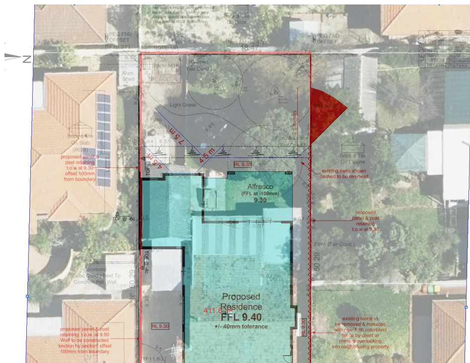
Figure 2 – Image depicting cone of vision (in red) from proposed alfresco to adjoining northern property.
