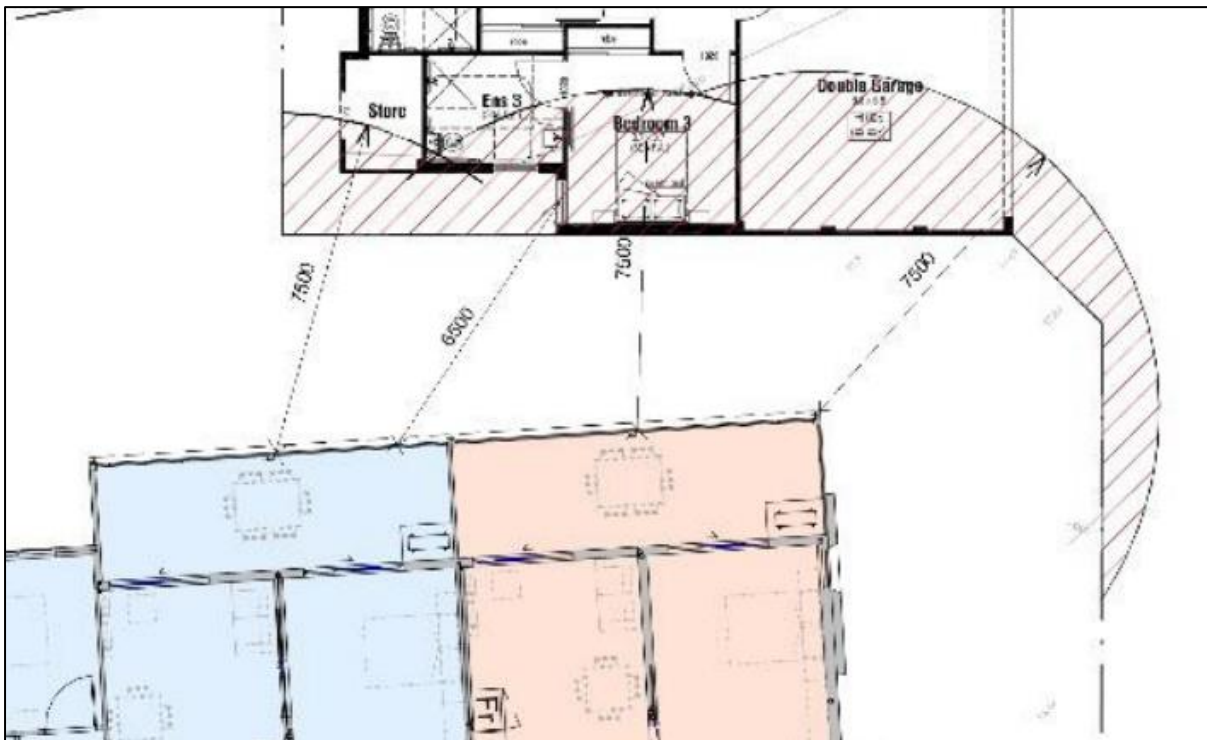
Figure 5 – Image depicting the intended building layout of the future grouped dwelling development. The overlooking from the balconies will fall within non-habitable spaces and a future driveway access leg.
