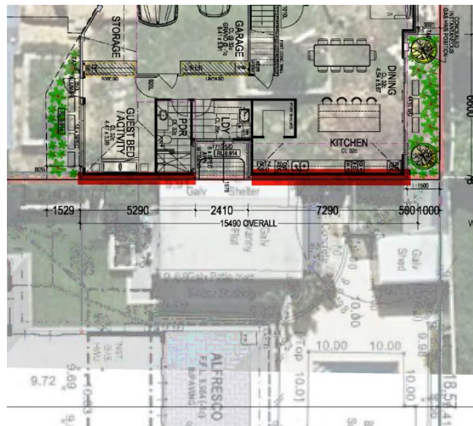
Figure 2: Ground floor plans of the proposal in relation to the neighbouring property at 24 Evershed Street. The parapet walls highlighted in red
