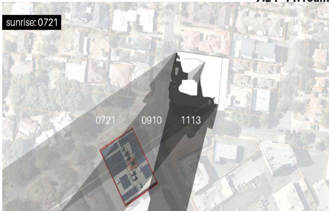
Figure 10: Shadow diagram indicating the time period overshadowing onto 1-7 Sleet Road, Applecross, would occur at winter solstice
