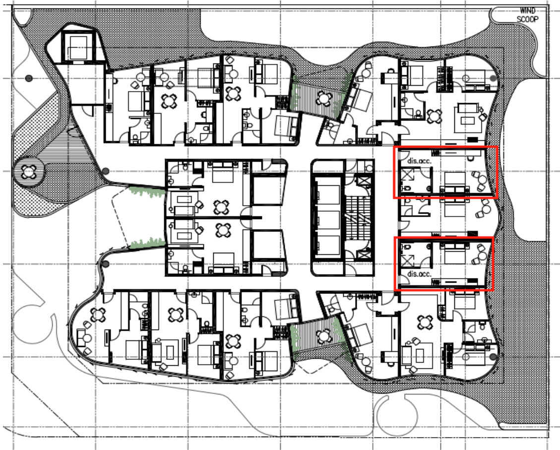
Figure 20: Proposed Level 2 with 15 short stay accommodation units comprising 5 x studio, 5 x 1 bedroom and 5 x 2 bedroom units. 2 units now provided as diable accessible units as marked in red
