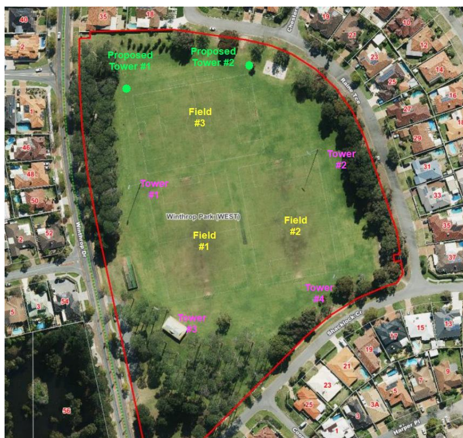
Figure 2: location of existing and proposed floodlighting towers.
