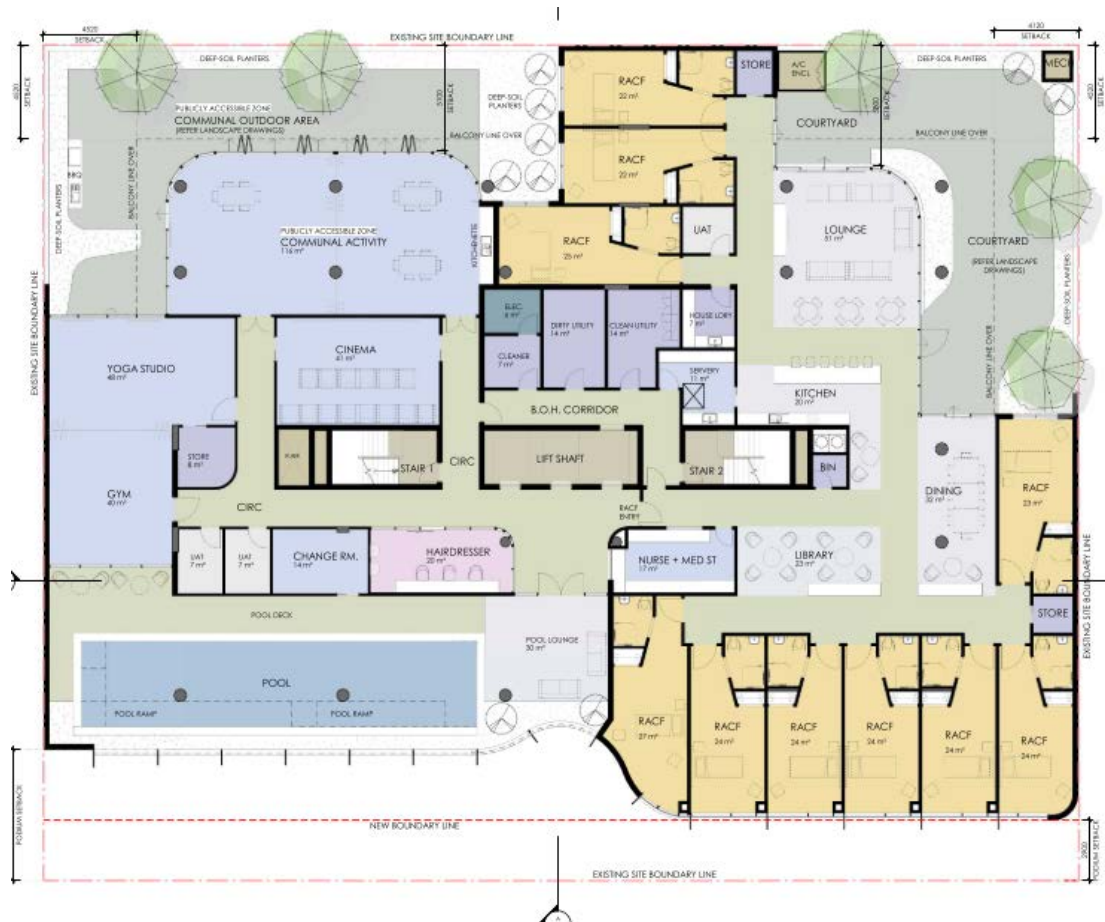
Figure 8: Level 2 floor plan with communal facilities including communal activity and outdoor areas, yoga studio, cinema and gym
