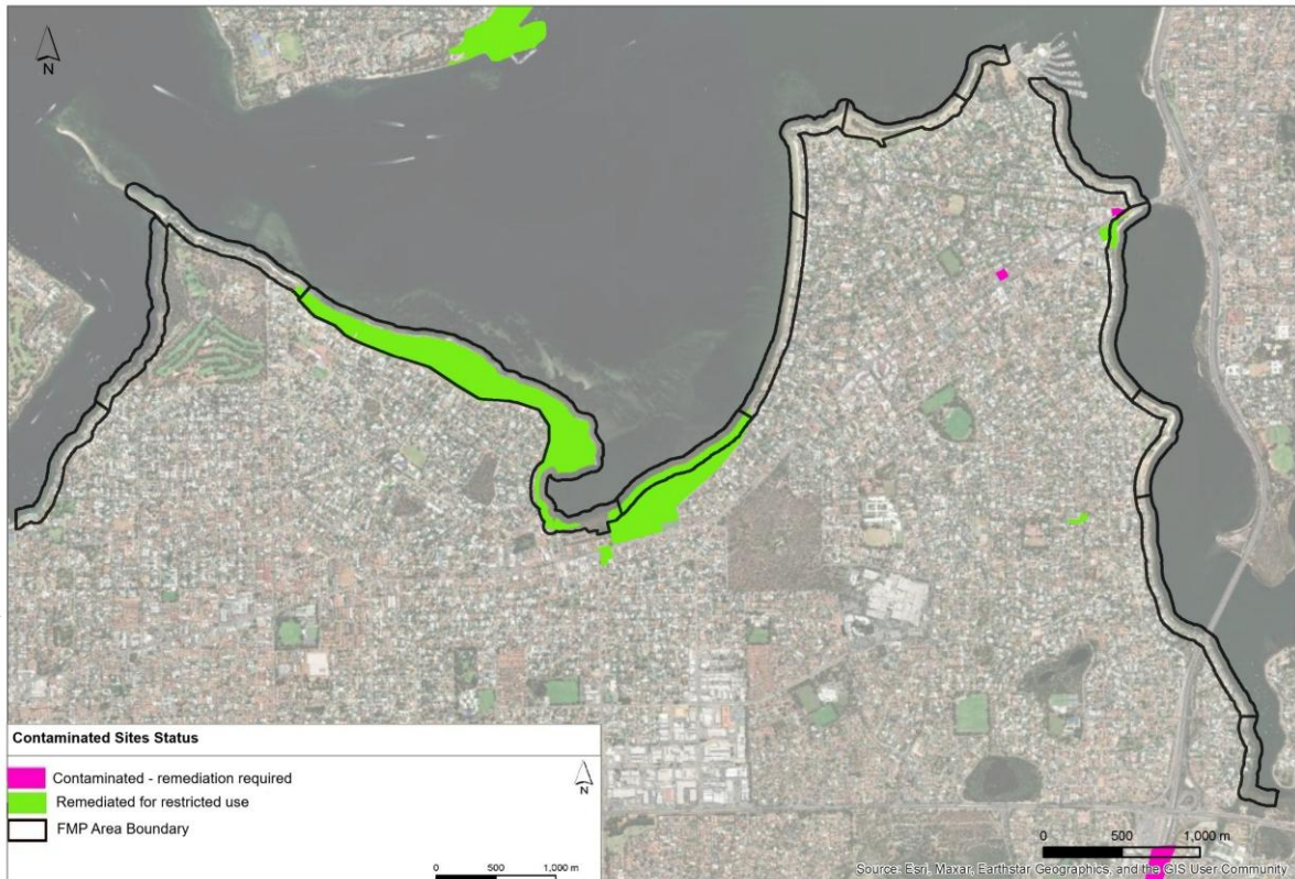
Figure 7. Location and extent of contaminated sites associated with the foreshore.
