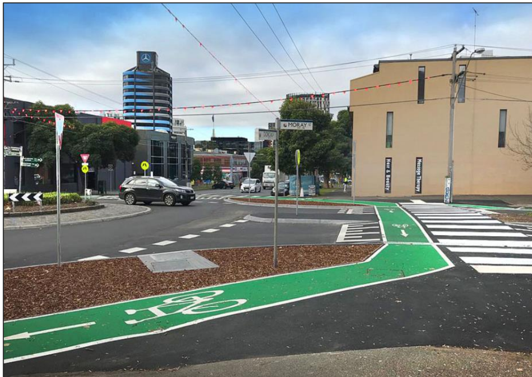
Figure 5-3: Roundabout Priority Crossing Points Set Back from the Entry (Moray Street/Dorcas Street, Melbourne)
