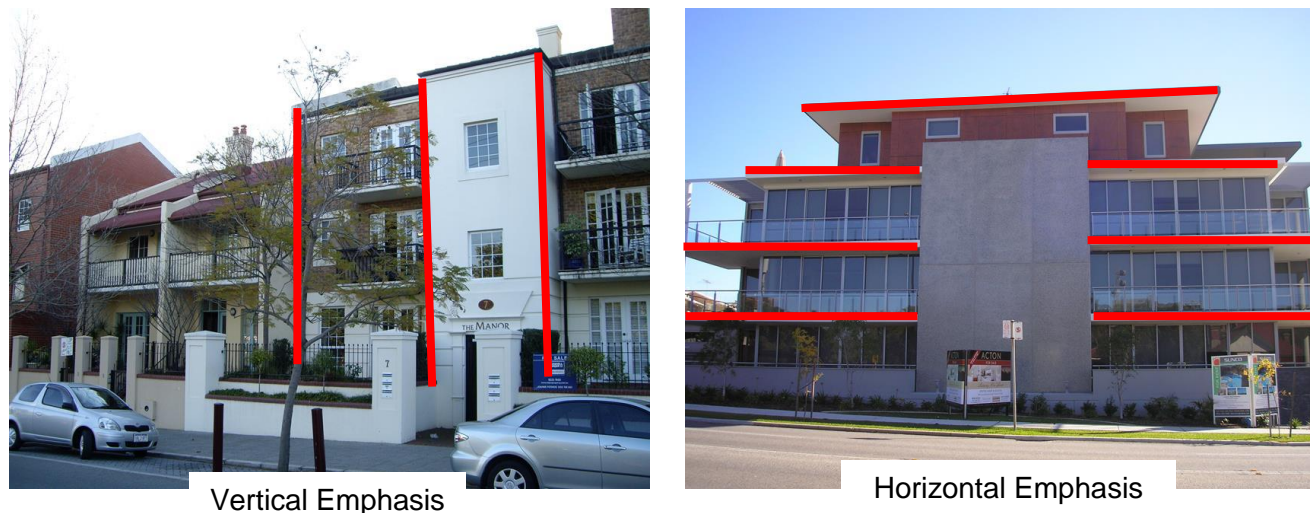
Figure 4 - Examples of Vertical and Horizontal Emphasis
