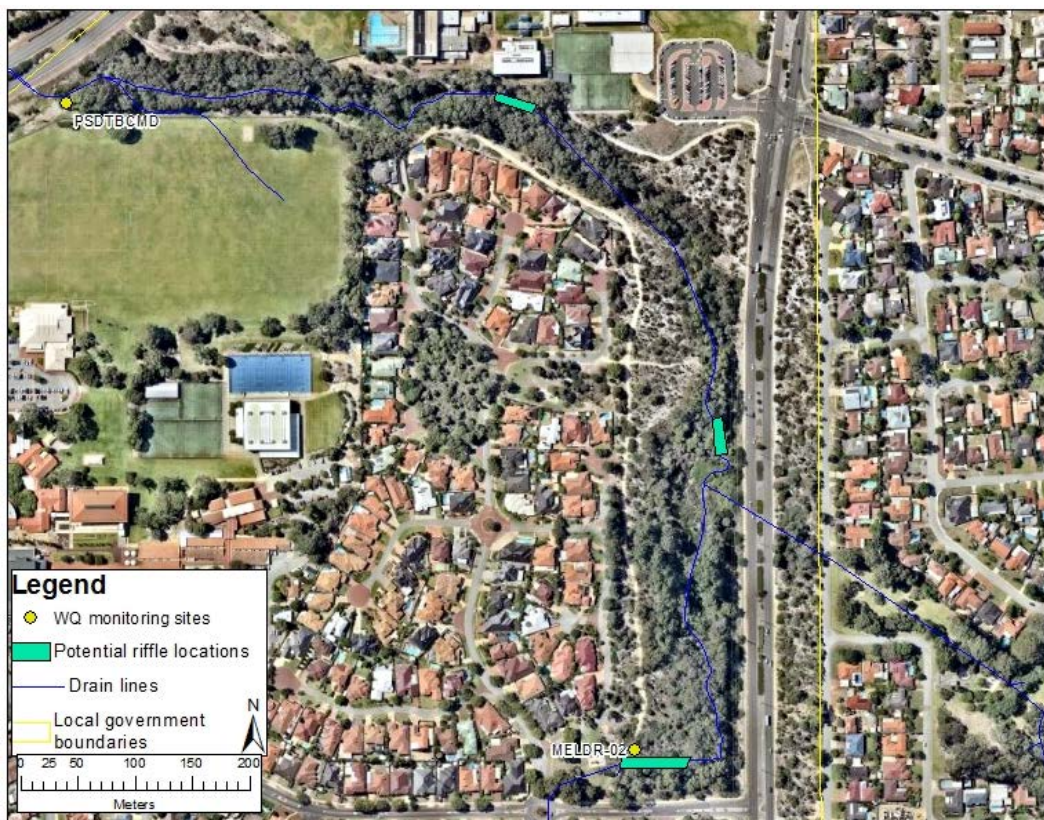
Figure 11.1-1: Approximate potential location riffles could be installed in Bull Creek.
