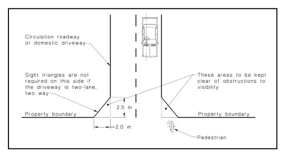
Figure 14 - AS 2890 Requirements for Pedestrian Sight Lines
