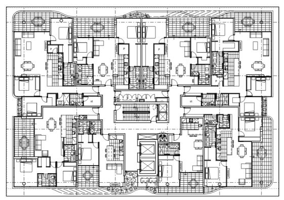
Figure 2: Proposed typical apartment floor layout.
