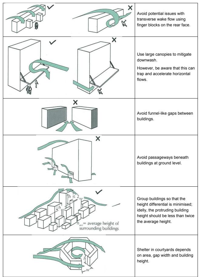
Figure 6 – Examples of wind flow around buildings and how to minimise the impact
