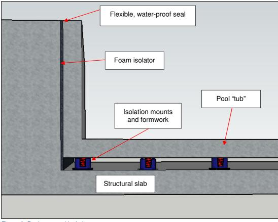
Figure 8: Pool structural isolation
