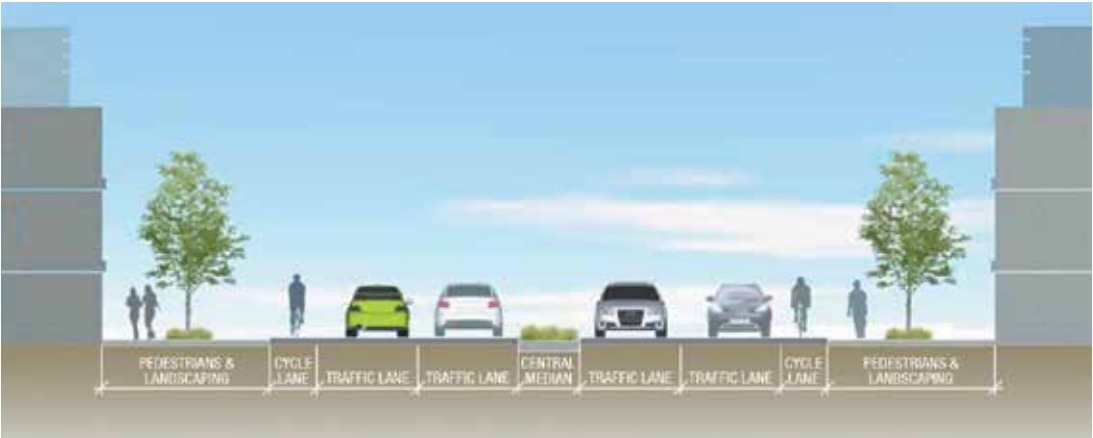
Figure 17 Indicative cross section – Manning Road
